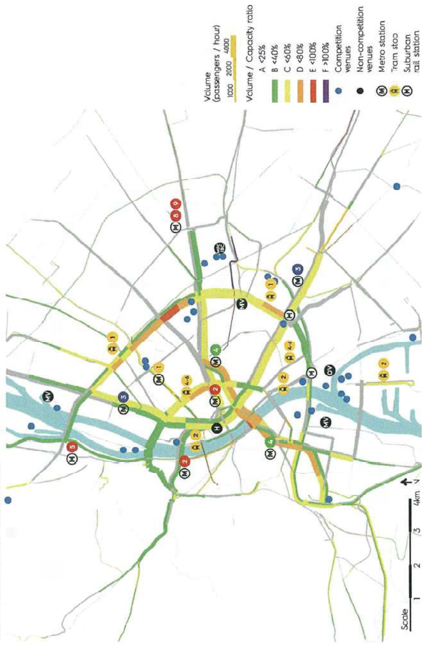
FIGURE 6 - LOADING OF PUBLIC TRANSPORT SYSTEMS DURING THE AFTERNOON RUSH HOUR OF THE BUSIEST DAY OF THE GAMES (DAY 11, 17:00 - 18:00)
